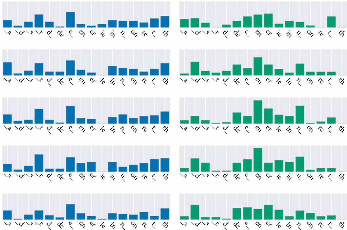
Figure 2.2: Character-bigram histograms for documents in English (left, blue) and German (right, green). Underscores denote spaces.
